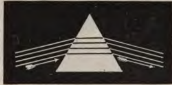
FIG. 146.—Passage of Parallel Rays Through a Prism.
